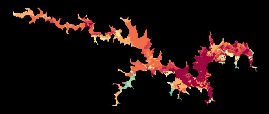
Water Quality (total suspended sediment) variability (2013 to 2017) along the Masinga Dam (near Nairobi, Kenya. These Data Cube results can be used to modify water sampling locations and timing with satellite data.
